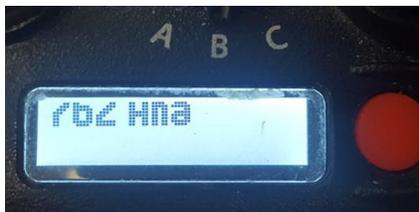
To avoid the potential for this to occur, a new version of Armada has also been developed to prevent firmware downgrades of new radios with the new display option set. If in the unlikely scenario that a new radio with new firmware has been misconfigured for the new top display, this display configuration can be corrected by changing the option in Tune/Test mode of the radio.
